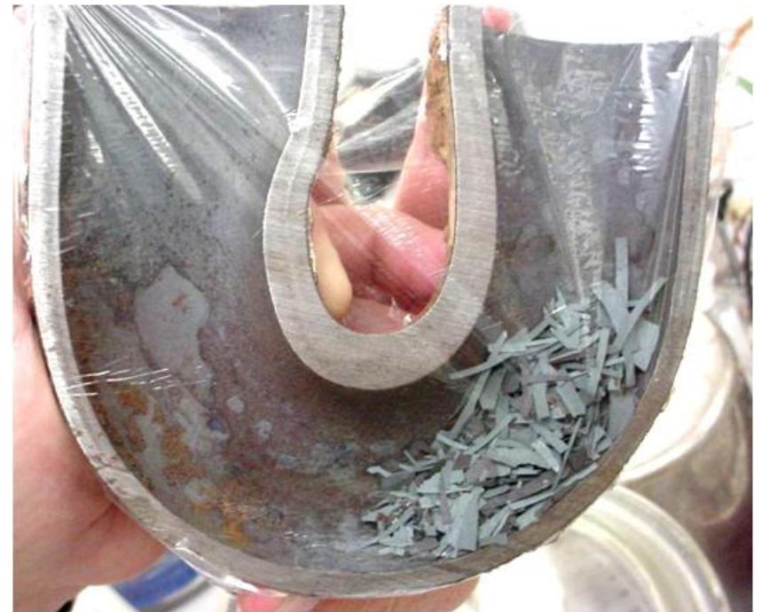
Exfoliated Oxide from 347H Tubing
